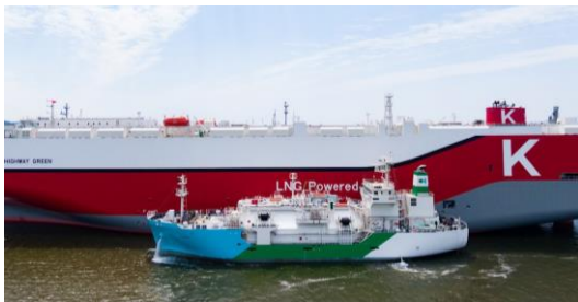
3,500m 3 type of LNG Bunkering Vessel [Kaguya] (Japan's First LNG Bunkering by ship-to-ship *Provided by CLMF)
